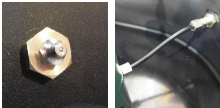
Grease lubrication system
