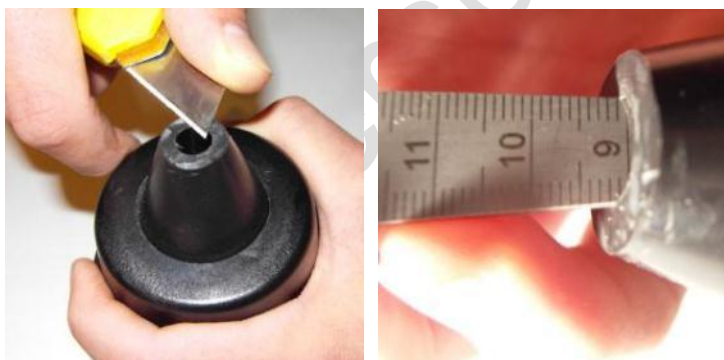
Cutting the jet to size and checking it with the taper gauge
